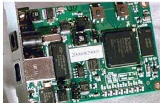
This Progeniq Bioblast accelerator card is used in some of the data collection for the quantitative portion of this report. Note that on the left of this PCI-compatible card, there is a power connector and a USB 2.0 port. Despite the low-performance interface (480 Mb/s), this card was able to provide about seven to 10x better performance than the pure software version of the HMMER application (a popular tool for nucleic acid and protein sequence analysis).
